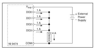
Figure 4. Increasing the Current to a Device Connected to the NI 9474
